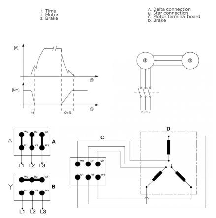
2. Separate brake power: the brake is powered off a terminal block separate from the motor's block; in this case t  $_1$  and t depend only on the characteristics of the brake.
